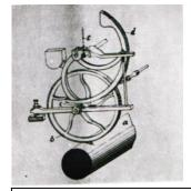
The mechanism of the 'Roller Machine'. The whole 'measuring wheel' lifts as the hide passes underneath and the cog engages the quadrant attached to the totaliser
