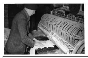
This photograph was featured in the last Edition and shows someone using a leather measuring machine in the UK, probably in the 1950's or 60's. This appears to be a 'Roller' type machine rather than a 'Pin Wheel' so we see that unapproved machines continued in use right up until the Regulations were discontinued.
