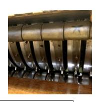
The 'Pin Wheel' measuring wheels, showing the sliding pins around the circumference. As each pin lifts it engages the cog on the shaft which operates the totaliser
